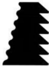
Reka Type-VI E/lg: 37.5/40.0 mm, Polymer: EPDM, Hardness: 55 +/- 5 Shore A
