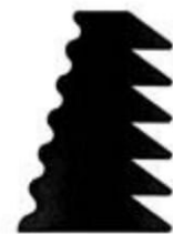
Reka Type-IV E/lg: 21/30 mm, Polymer: EPDM, Hardness: 70 +/- 5 Shore A
