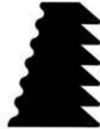
Reka Type-II E/lg: 22/30 mm, Polymer: EPDM, Hardness: 55 +/- 5 Shore A
