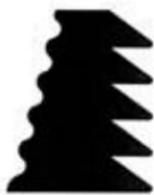
Reka Type-II E/lg: 20/25 mm, Polymer: EPDM, Hardness: 70 +/- 5 Shore A
