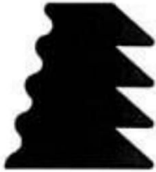
Reka Type-I E/lg: 18/20 mm, Polymer: EPDM, Hardness: 55 +/- 5 Shore A
