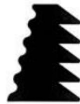
Reka Type-I E/lg: 19/25 mm, Polymer: EPDM, Hardness: 70 +/- 5 Shore A
