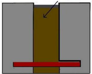
Deesa Jolly Board is brought flush with the concrete slab and extends full depth of the slab, placed approximately ¾ of an inch below the surface of the concrete slab. A suitable sealant is applied either at the top or bottom of the slab to close the joint against hydrostatic pressure. The dowel bar is used to preserve alignment of adjacent sections of concrete slab. Deesa Jolly Board is fabricated to receive dowel bars and the entire joint assembly is placed in position before pouring concrete.
